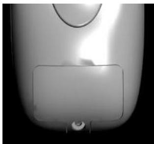
As the battery discharges, the performance (RF range) of your remote controller gets shorter. It is necessary to replace the battery. You will recognize the weak battery according to a very weak tone when your transmitter is turned on or off. Prepare a spare 3V lithium battery CR2450 and follow the previous section on Installation of the battery in the remote controller.
